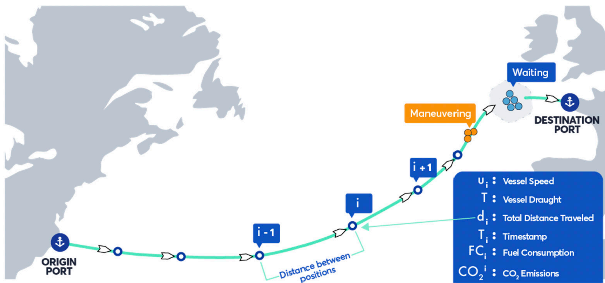
Figure 1: Construction of voyages from origin port to destination port. Source: MarineTraffic collection.
