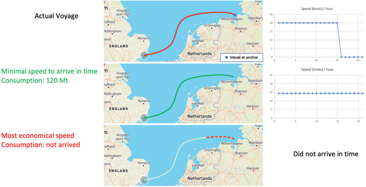
Figure 3: Understanding JIT speed (minimal speed to arrive in time)
