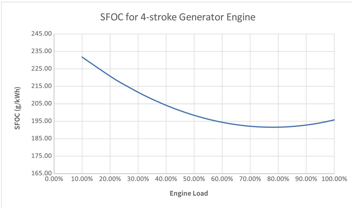
**Figure 4:** Indicative specific fuel oil consumption (SFOC) for a four-stroke engine
