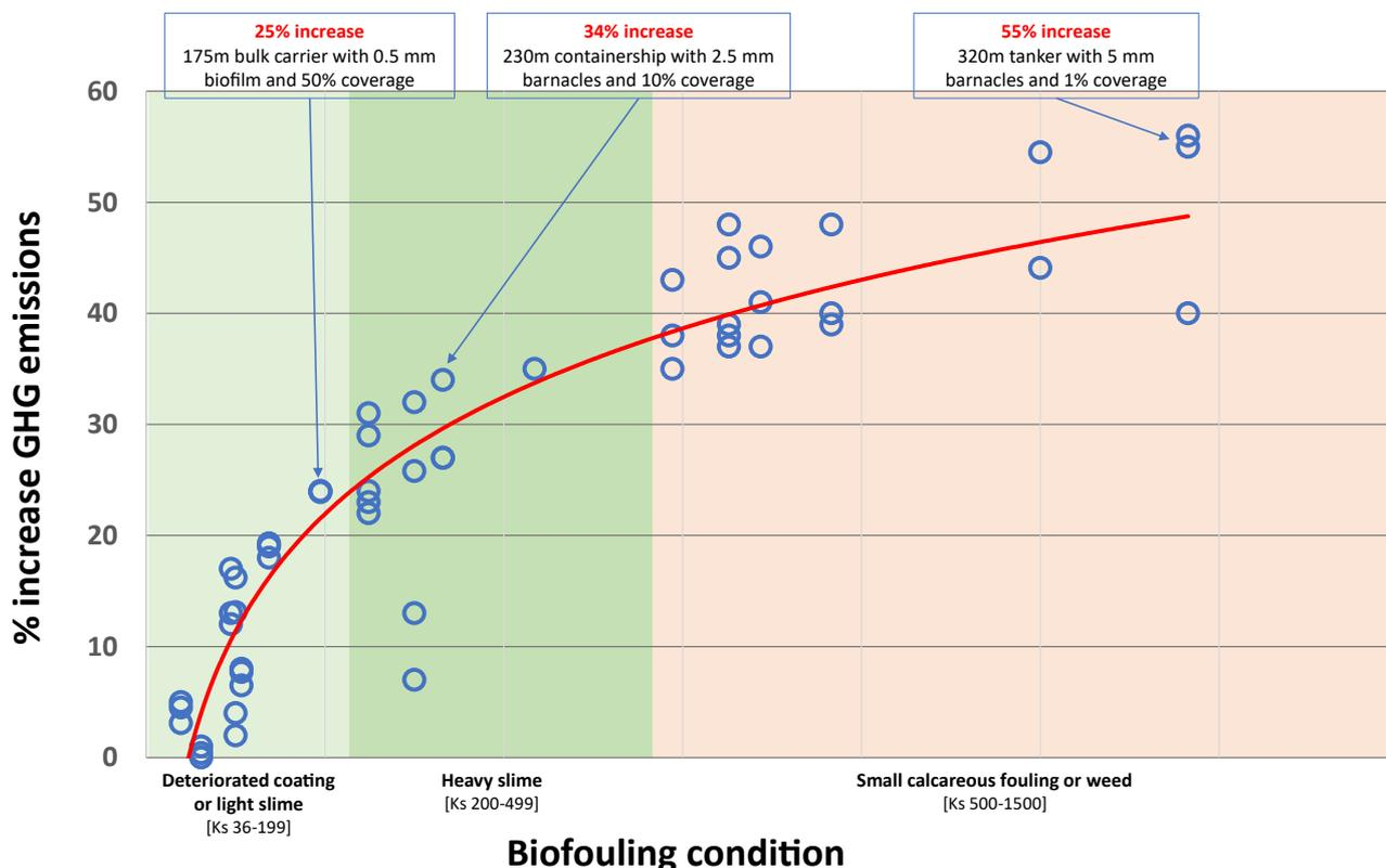
**Figure 3:** *Impact of ship hull biofouling on GHG emissions (data and analysis from GloFouling Partnerships Project)*
