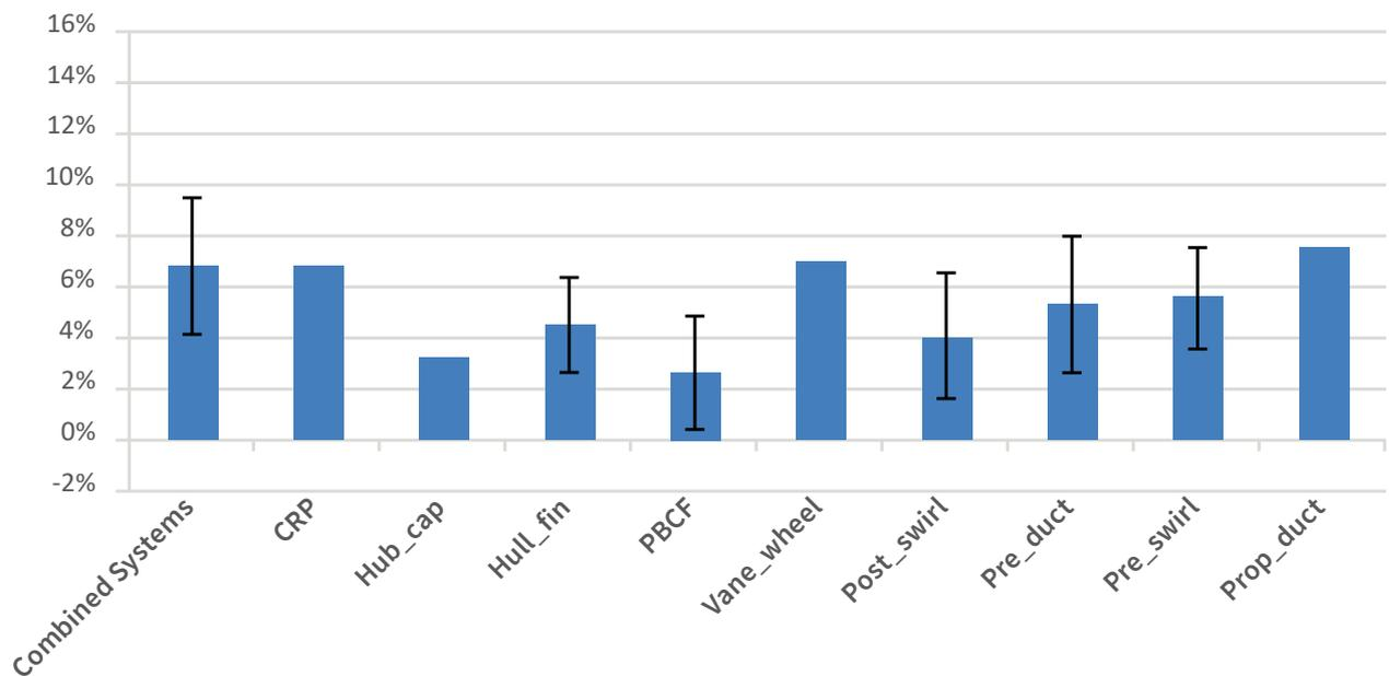
**Figure 5:** Average energy saving ratio and standard deviation for a range of EETs (data and analysis by GRIP project)
