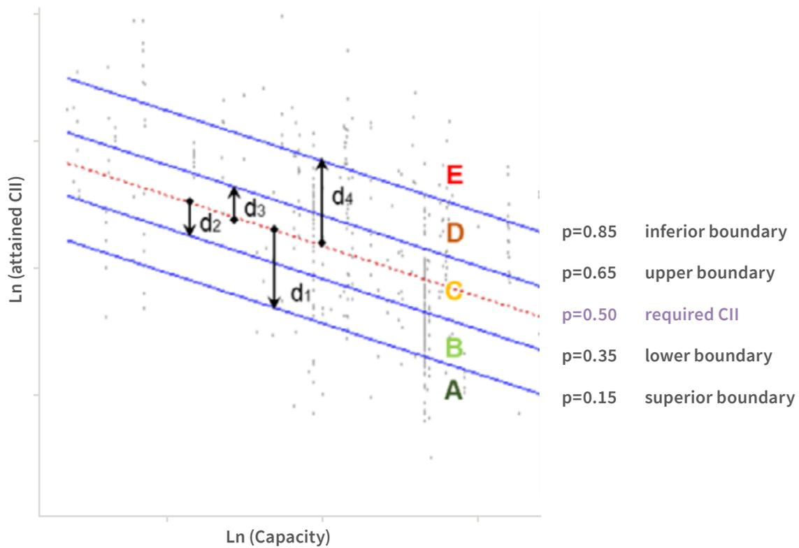
**Figure 7:** Illustration of CII rating boundaries from the 2021 Guidelines on the operational carbon intensity rating of ships (CII rating guidelines, G4) (resolution MEPC.339(76))
