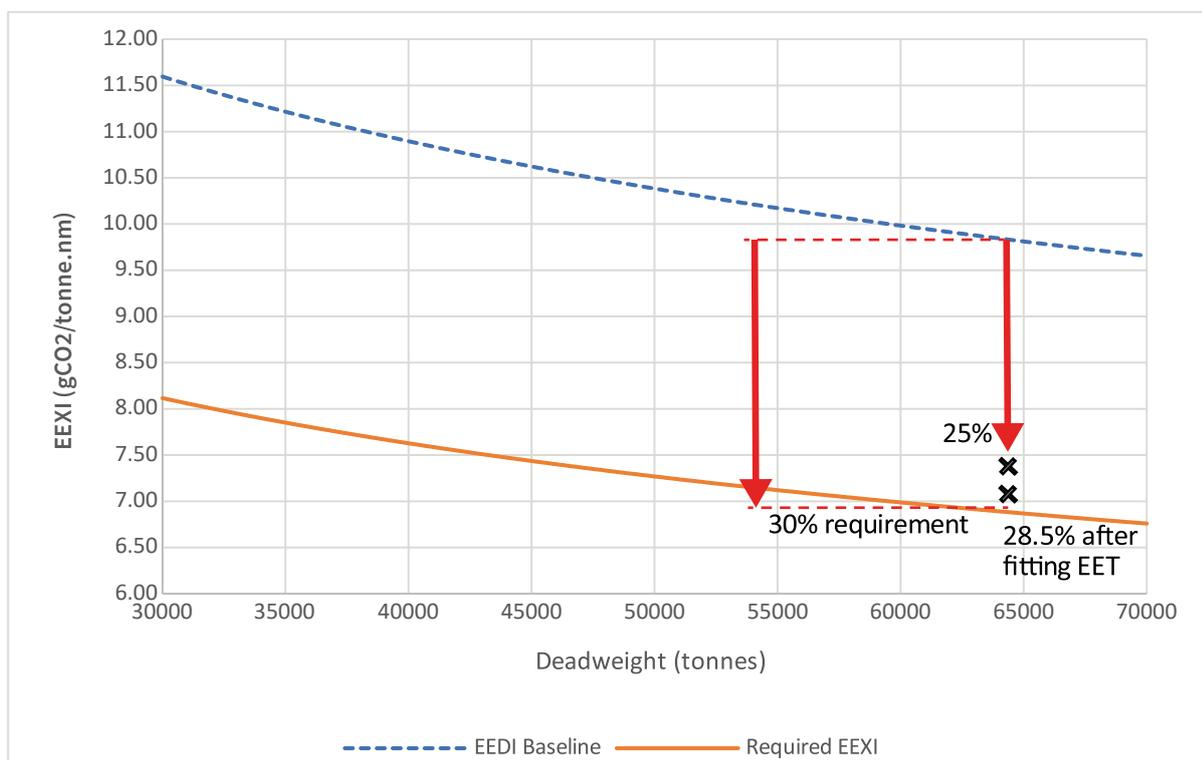
Figure 6: Effect on attained EEXI value when retrofitting an EET
