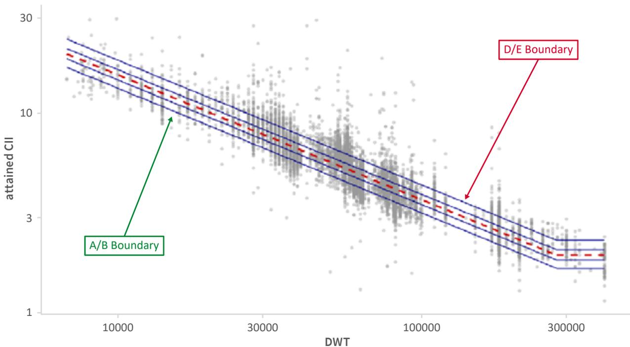
**Figure 8:** CII scatter and rating boundaries for bulk carriers from “Reduction of GHG emissions from ships: technical report on CII guidelines development” (document MEPC 76/INF.10)
