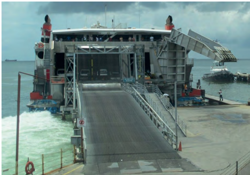
Figure 4: T&T SPIRIT berthing with stern at car ramp and passenger ramp in Port of Spain ferry terminal
