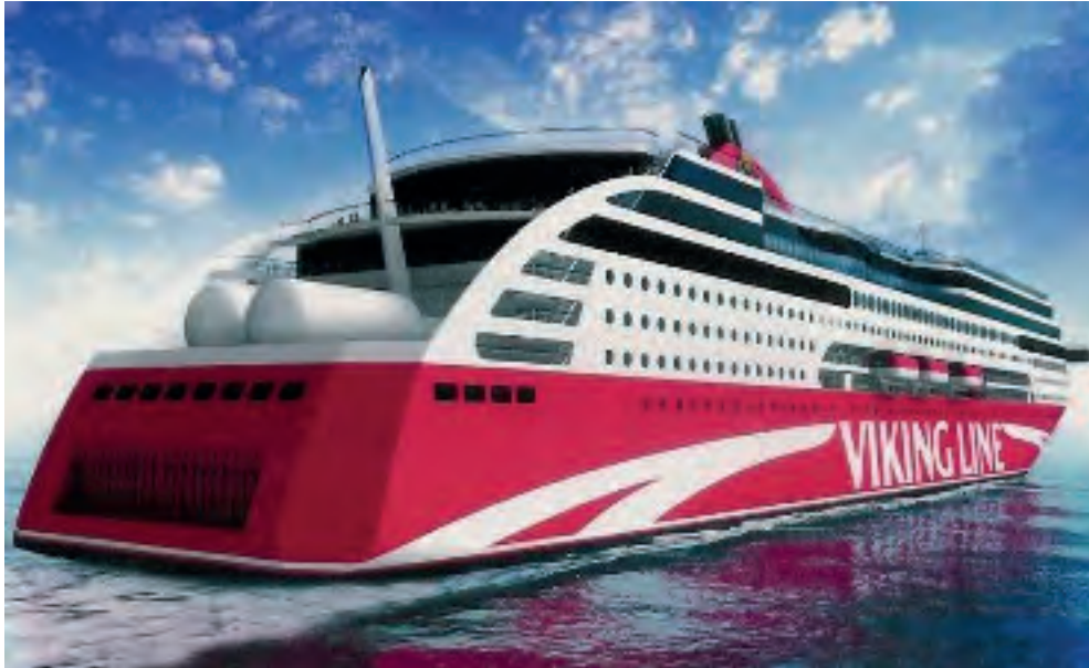
Figure 20: VIKING GRACE with external LNG tanks (Image reproduced courtesy of Marine Insight.com)
