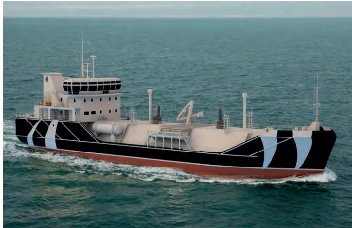
Figure 23: A 2 800 m 3 LNG bunker vessel (Photograph reproduced courtesy of White Smoke Shipping)
