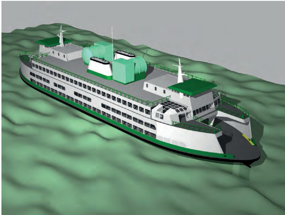
Figure 24: Rendering of LNG tanks on an Issaquah class (Image reproduced courtesy of WSF)
