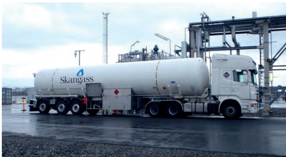
Figure 26: A typical European Truck/LNG Semi-trailer combination (Photograph reproduced courtesy of Skangass AS)
