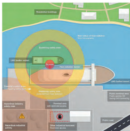
Figure 41: Schematic illustration of how a credible design LNG leakage scenario is used for input to model calculations of gas dispersion and heat radiation from associated fire scenarios
