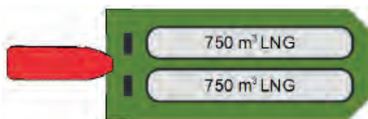
Figure 33: Sketch of a 1\,500\text{ m}^3 LNG barge connected to a harbour tug
