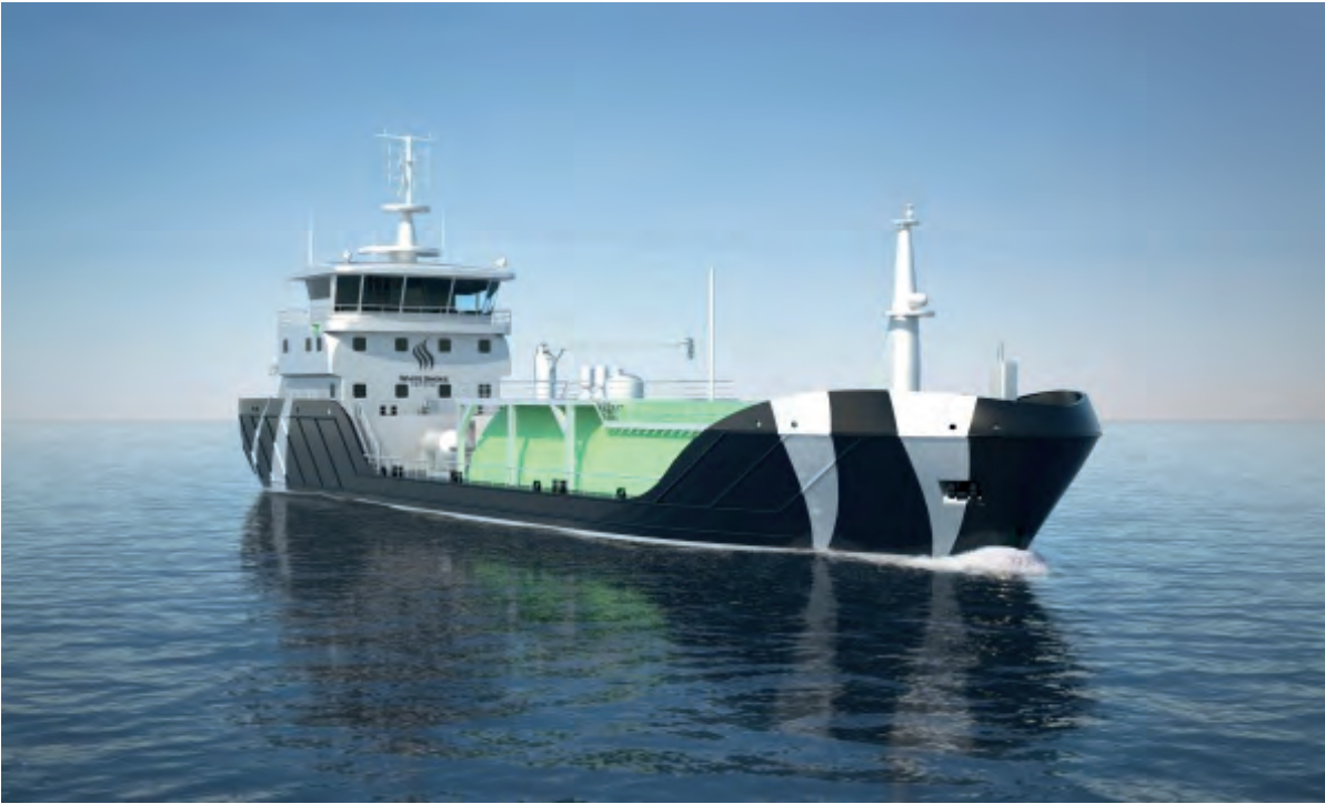
Figure 50: Proposal for 1 400 m 3 LNG bunker vessel
