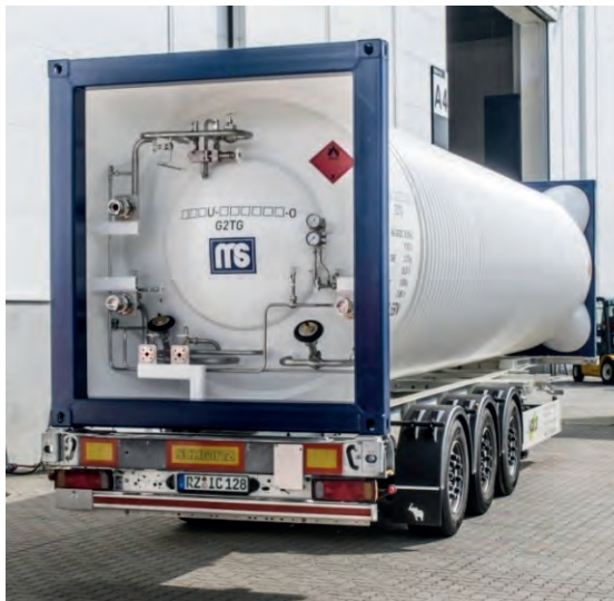
Figure 24: LNG fuel container (Photograph reproduced courtesy of Marine Service GmbH)
