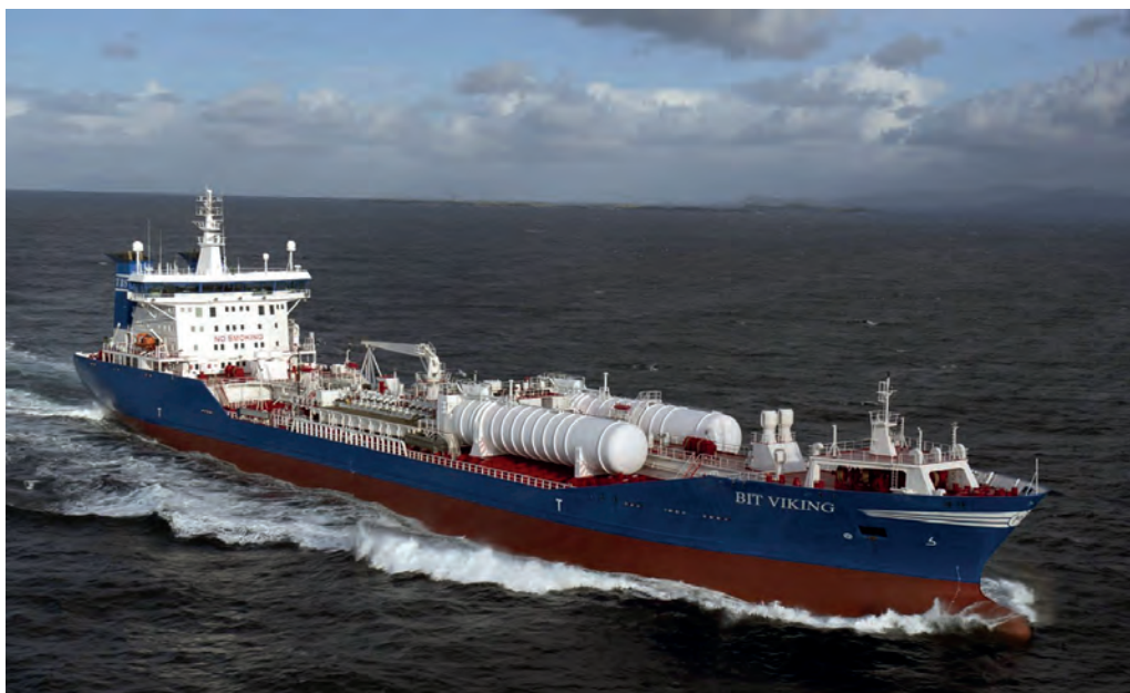
Figure 10: BIT VIKING LNG fuelled product tanker
