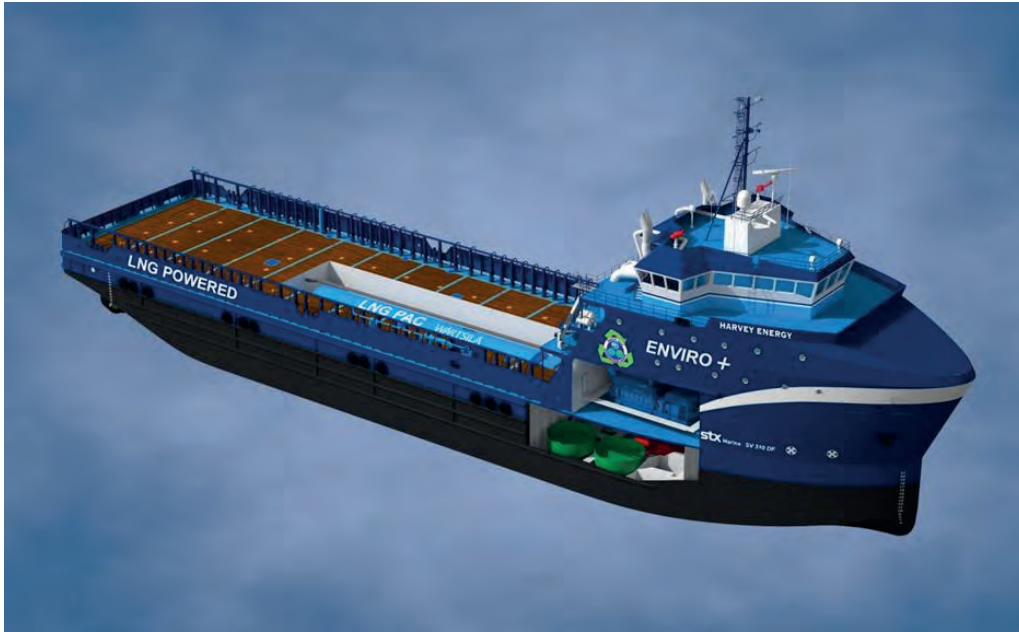
Figure 18: An illustration of Harvey Gulf's LNG powered OSVs (Image reproduced courtesy of Harvey Gulf)
