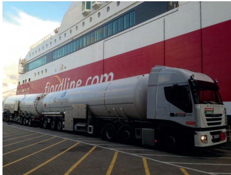
Figure 21: Truck to ship bunkering (TTS) of LNG from two trailers in parallel (Photograph reproduced courtesy of Skangass AS)
