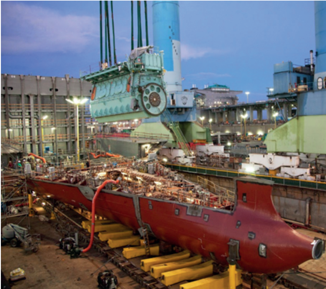
Figure 2.1: Installation of first dual-fuel slow speed engine MAN 8L70ME-C8.2GI, TOTE
