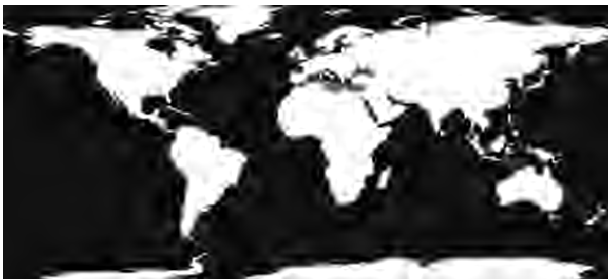
Figure 2: Sea region definition illustration. GIS shapefile has been read by the pre-processor. The resolution of the sea region mapping is 0.1 \times 0.1 degrees
